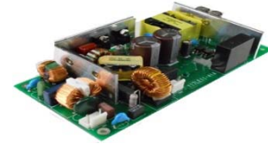
Embedded power supply module
