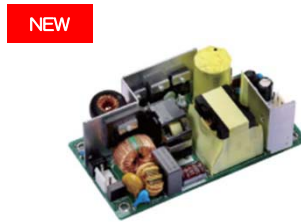
SW Power Supply
